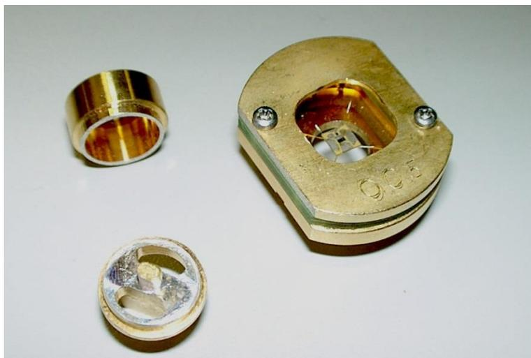
Figure 2-11. DR Heat Capacity Sample Mount and Accessories
