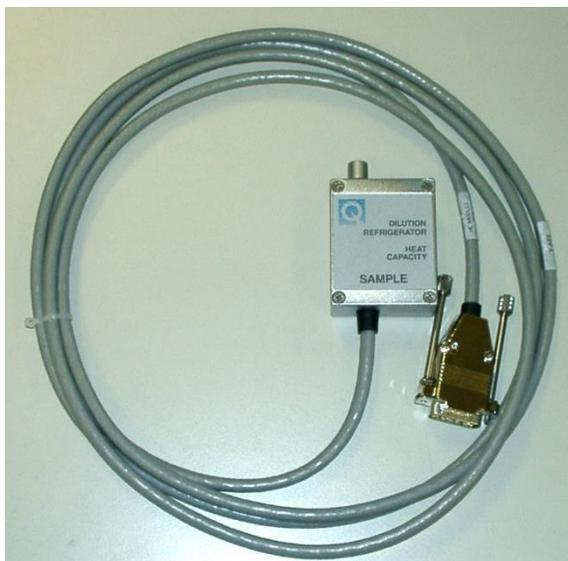
Figure 2-13. DR heat capacity option cable
