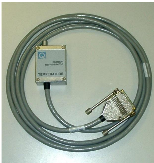
Figure 2-7. Temperature control cable
