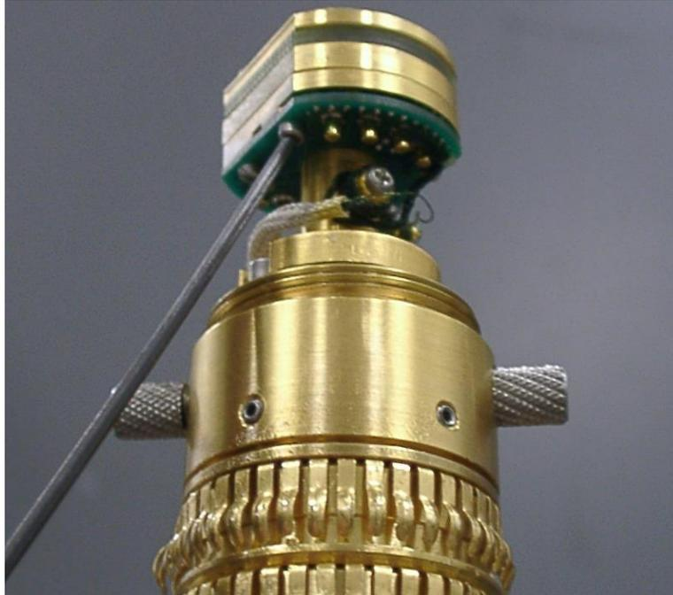
Figure 4-3. Tighten hex screws on sample stage.
